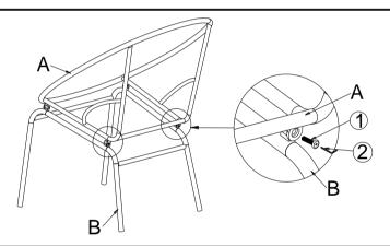
Attach Chair Part(A) to Leg Part(B) using Bolts(1) with Allen Key(2).
