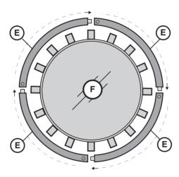
Lay down all 4 sections of the Support Tubes (E) & Fabric Seat (F) like the illustration shown above.
