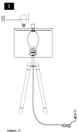
Step 2 Insert the bulb(H) into the socket(D).
