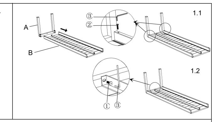
Open the carton and place all the parts onto a clean, non-marring surface. Insert Leg(A) into Seat(B) as pictured above.
