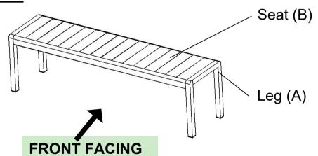
This Bench has multiple parts and may require up to 20 minutes to assemble. To give you an overview of the bench parts, the above picture is to help you put the various parts into perspective. Please read through the instructions below to familiarise yourself with the parts and steps before assembly.
