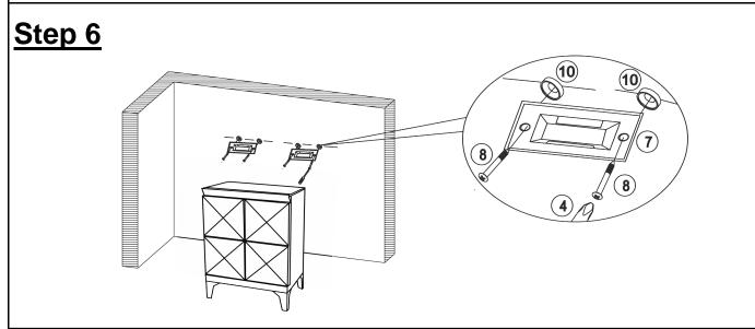
Attach Brackets (7) to Wall Plugs (10) using Wall Plug Screws (8) with Screwdriver (4).
