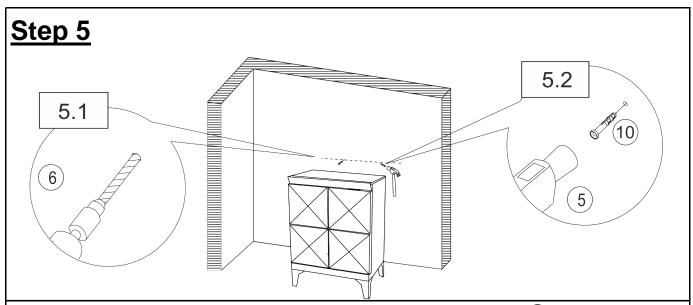
5.1 Drill two holes on wall at same height as Brackets (⑦) on Cabinet with Power Drill (⑥).
