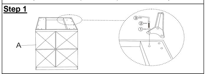
With assistance from your adult partner, place the Wooden Cabinet (A) face down as picture, on a clean, non-marring surface. As shown in "Step 1" picture attach Metal Leg (B) to Wooden Cabinet (A) using Washers (1) Bolt (2) with Allen Key (3).
