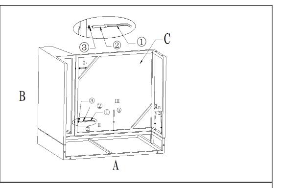
Attach Seat(C) between the Left Armrest(A) and Chair Back(B) using Bolt(2) and Washer(③) with Allen Key(①) from position # I to # V as shown above. Do not fully tigthen.
