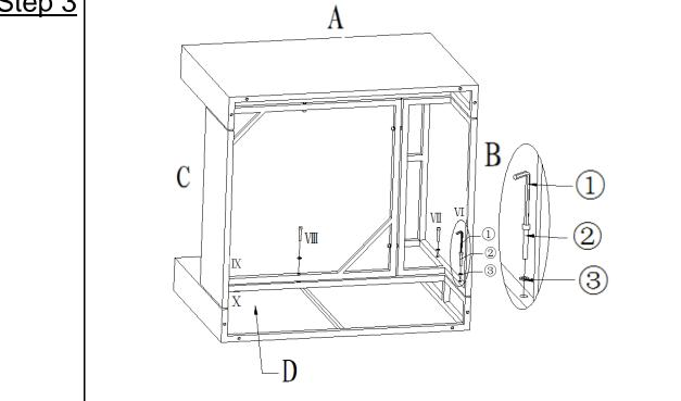
Attach Right Armrest(D) to the Chair Back(B) and Chair Seat(C) using Bolt(2) and Washer(③) with Allen Key(①) from position # VI to # X as shown above. Do not fully tigthen.
