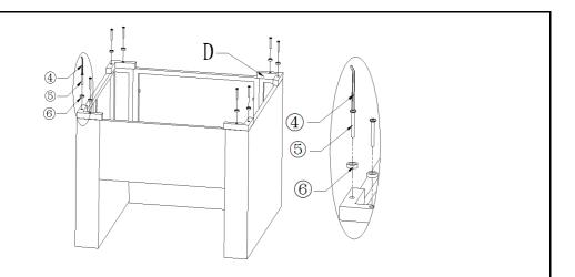
Attach the Feet(D) to the Chair using Bolts(5) and Washer Rings(6) with Allen Key(4).
