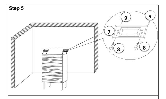
Attach Brackets 7 to Wall Plugs 9 using Wall Plug Screws 8 with Screwdriver 4.
