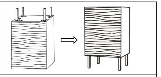
Repeat "step 1" to assemble another leg(B) to Badside (A). Upon assembly of all the legs, flip the Chest as shown in above picture.
