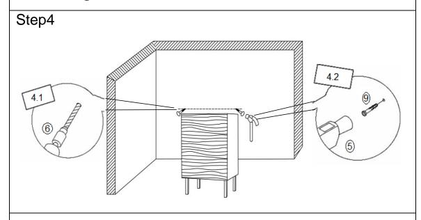
4.1) Drill two holes on wall at same height as Brackets  $\bigcirc$  on Chest with Power Drill  $\bigcirc$  .
