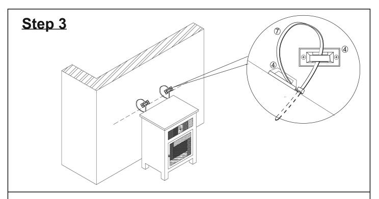
Move Bedside to the wall. Pull the Restraint Straps (7) through the Brackets (4) on the wall and Bedside one by one, and pull the Restraint Straps (7) tight.
