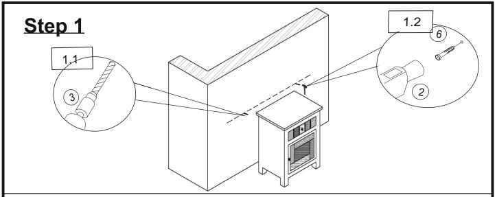
1.1) Drill two holes on wall at same height as Bracket (4) on Bedside with Power Drill (3).
