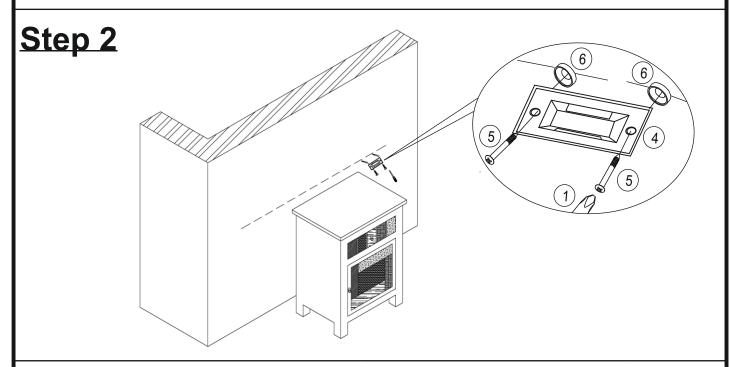
Attach Brackets (4) to Wall Plugs (6) using Wall Plug Screws (5) with Screwdrivers (1)
