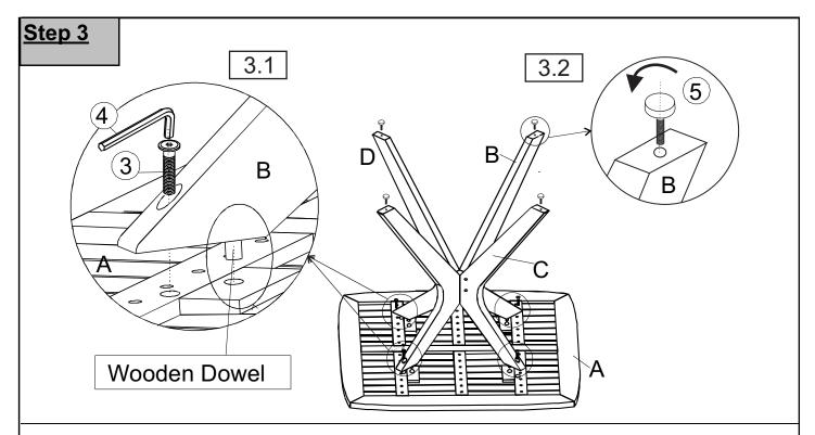
**3.1)** Place Table Top (A) facedown onto a clean, non-marring surface to avoid any scratches or damage to the product.
