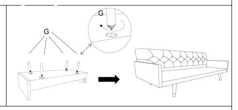
Install the Wood Legs(G) at the bottom of the Sofa by placing one Gasket(⑦) on the threaded stem.
