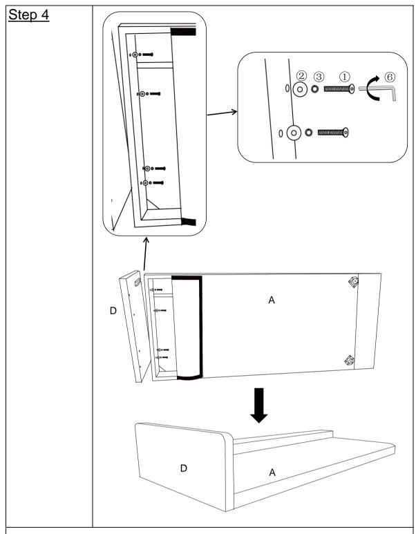
Align Left Arm Board(D) on the left side of the Sofa Base(A). Attach Left Arm Board(D) to Sofa Base(A) using Bolts(①) Spring Washers(③), and Washers(②) with Allen Key(⑥).
