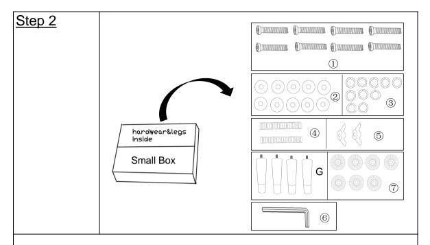
Open the Small Box and take out the Wooden Legs(G), Gaskets( $\Im$ ), Bolts( $\Im$ ), Washers( $\Im$ ), Spring Washers( $\Im$ ), Double-threaded Bolts( $\Im$ ), Wing Nuts( $\Im$ ), and Allen Key( $\Im$ ).
