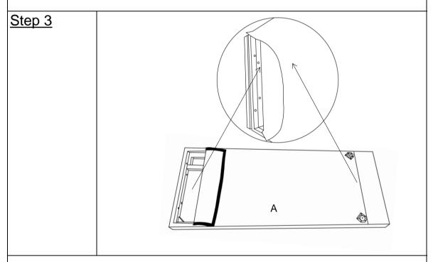
Carefully peel back the left and right non-woven cover under the Seat Base(A) to expose the mounting positions.
