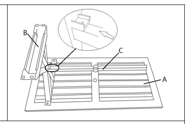
Insert the Support Rod(C) into the Table Leg with pre-attached Leveller(B) as pictured.
