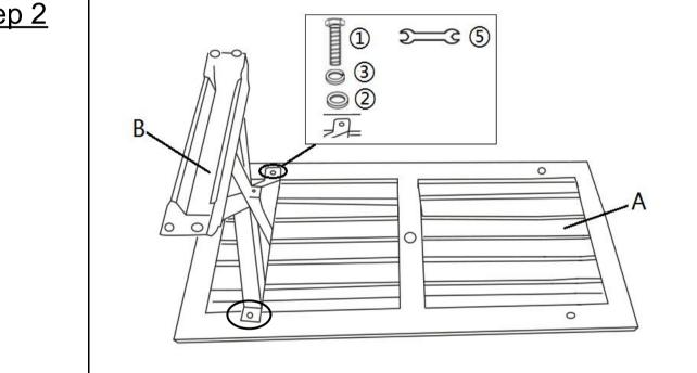
Lay the Table Top(A), facedown onto a flat, clean, non-marring surface. Attach Table Leg with pre-attached Leveller(B) to Table Top(A) using Washers (2), Spring Washers(3), and Hex Bolts(1) with Spanner(5).
