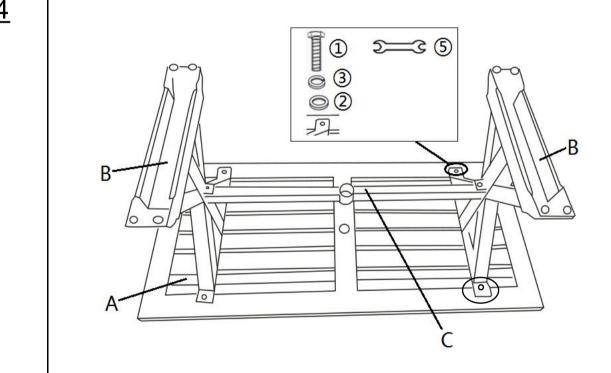
Insert the Support Rod(C) into the other Table Leg with pre-attached Leveller(B). Then attach the Table Leg with pre-attached Leveller(B) to Table Top(A) using Washers(2), Spring Washers(3), and Hex Bolts(1) with Spanner(5). **Do not fully tighten the Bolts.**
