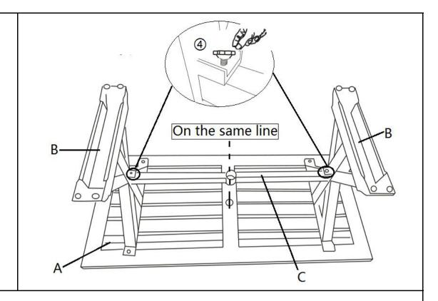
Align the mounting position on Table Leg with pre-attached Leveller(B) to Supporting Rod(C).
