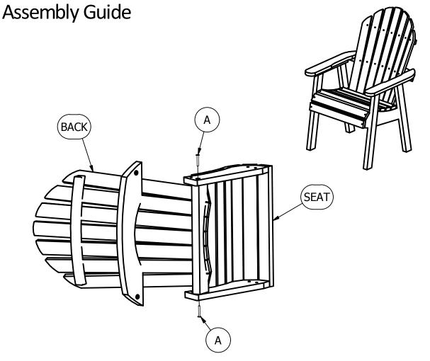
**1)** Insert (1) "A" Bolt into Lower Hole on Each Side to Attach Seat to Back. Make Sure the Back is Fully Upright. Make Bolts Snug, but Do Not Overtighten.
