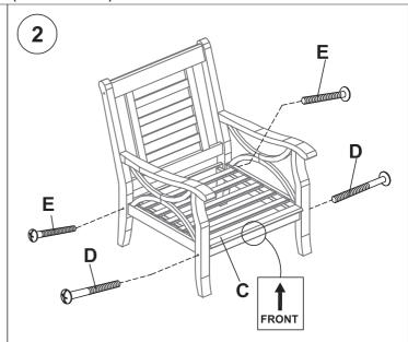
Attach the seat (C) into right and left side frames (A1 & A2). Secure using 2" bolts (D) and 1 1/2" bolts (E), as shown.
