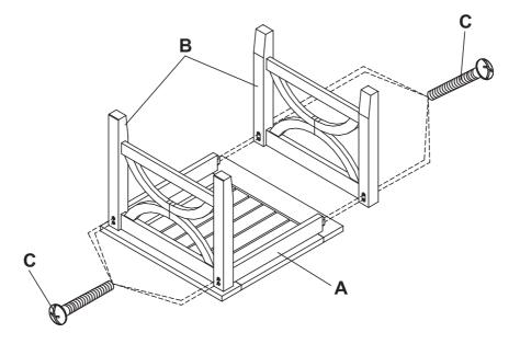
Attach the leg frame (B) to the table top (A) and secure with 1 1/2" bolts (C). Using phillips screwdriver.
