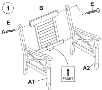
Attach back support (B) into right and left side frame (A1 & A2) to the matching holes. Secure using 1 1/2" bolts (E), as shown.
