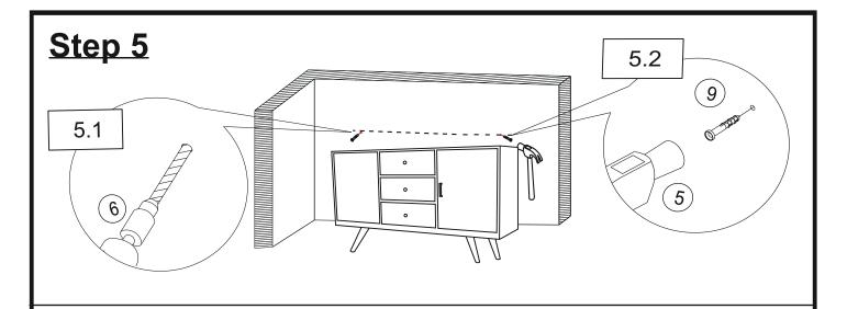
5.1) Drill two holes on wall at same height as Bracket (7) on Sideboard (A) with Power Drill (6).
