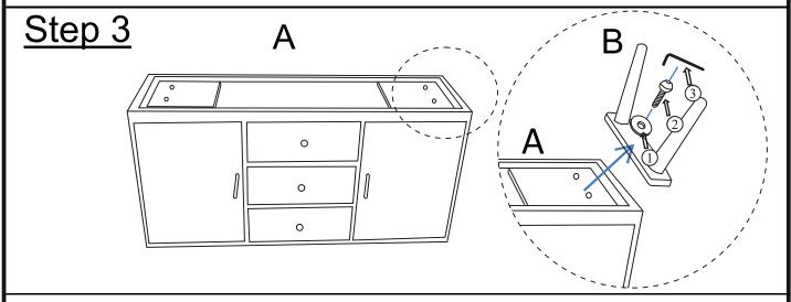
With assistance from your adult partner, place the Sideboard Top (A) face down as picture on clean surface. As shown in "Step3" picture attach Leg (B) to Sideboard top (A) using Washer (①), Bolt(②) with Allen key (③). Repeat "Step3" to assemble the other Leg (B) to Sideboard top(A)
