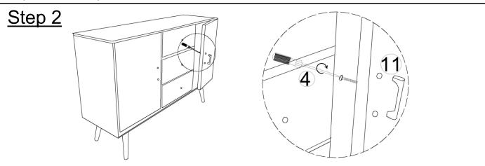
Install the Handle (1) on the door with the help of Screwdriver (4) as the pictured above. Repeat the step for all the door.
