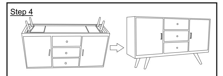
Upon assembly of all the legs, flip the Sideboard as shown in (Step 4).
