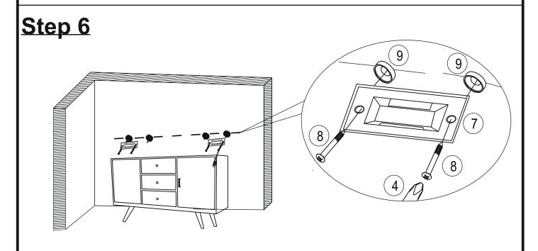
Attach Brackets (⑦) to Wall Plugs (⑨) using Wall Plug Screws (⑧) with Screwdrivers (④)
