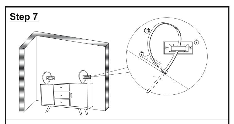
Move Sideboard to the wall. Pull the Restraint Straps (®) through the Brackets (⑦) on the wall and Sideboard one by one, and pull the Restraint Straps (⑦) tight.
