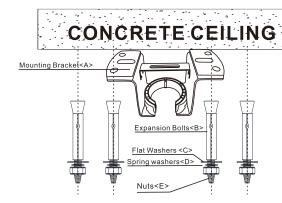
Note: According to the ceiling of different materials, use different screws to fix the hanging bracket. Don't fix the hanging bracket on the wood ceiling less than 12MM to prevent danger caused bloosening of screws.
