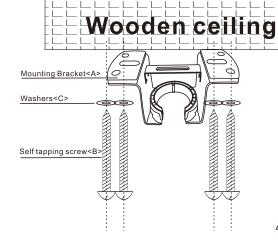
For wooden ceiling, use wood screw to drill on the wooden beam or the "junction box" to fix the hanging bracket (selection is made according to actual requirements of the customers).
