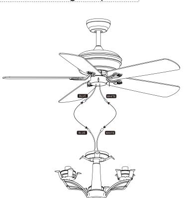
CAUTION:To reduce the risk of electric shock, disconnect the electrical circuit to the fa before installing the light fixture.
