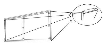
Take out the silders in the four ends of Table Top Frame(C) using Allen Key(3).
