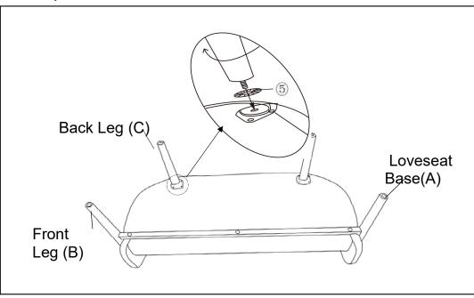
Install the Back Leg(C) at the bottom of the Chair by placing one Gasket(⑤) on the threaded stem. Then insert threaded stem into the threaded mounting postion at the corner of the Chair. Tighten by turning the Leg clockwise.
