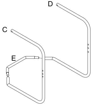
Step 3. Attach support legs (parts C & D) to chair back (part A) and chair seat (part B) using long bolts (part #1), hex nuts (part #4), flat washers (part #5), plastic washers (part #8), wrench (part #6) and allen wrench (part #7).
