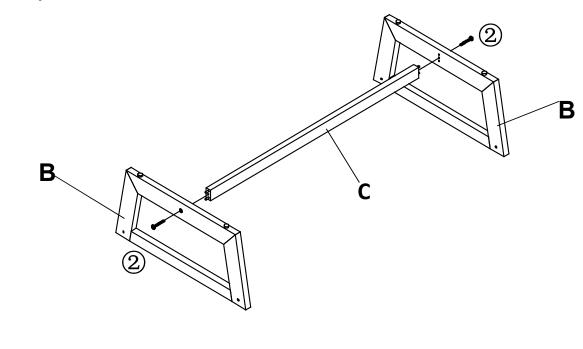
Place the Leg (B) and Coss bar (B) facedown as shown above.
