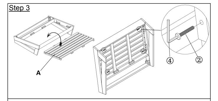
Insert Seat Panel (A) into assembled Bench I using Bolt (2) with Allen Wrench (4) as shown in picture above.
