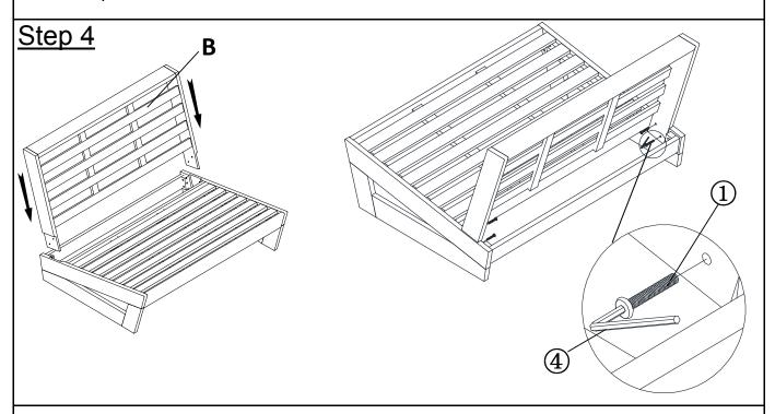
Insert tenons on Backrest Panel (B) into the mortises of Right Leg (C) and Left Leg (D) as shown above.
