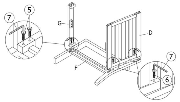
With the help of your adult partners, attached the tenons of Backrest Panel (D) and Support Bar (G) into the mortises of Left Panel (F) using Bolt ( $\bigcirc$ 5) and ( $\bigcirc$ 6) with Allen Key ( $\bigcirc$ 7) as shown in picture above. Repeat the same process with the Right Panel (E) **Do not fully tighten the Bolt.**
