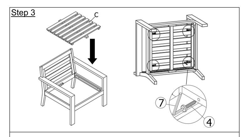
Insert Seat Panel (C) onto Chair frame as shown above by using Screw (4) and Allen Key (7).
