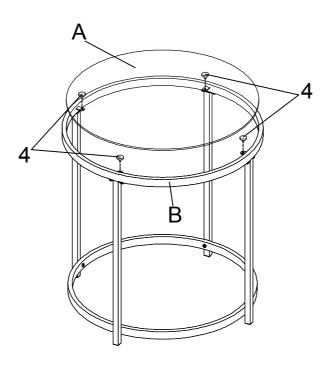
Step 3: 1.Insert Suction Cup (4) onto Top Frame (B) as shown. 2.Place the Glass (A) to the Suction Cup (4) as shown.
