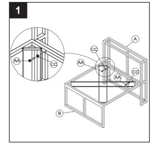
2. Align all four holes of the side frame (C). For each hole, insert M6 x 35 L bolt (AA) through M6 washer (CC), the seat frame (B) and back frame (A). Repeat this step for the oposite side. Do not tighten completely. Repeat this procedure for the adjacent hole.
