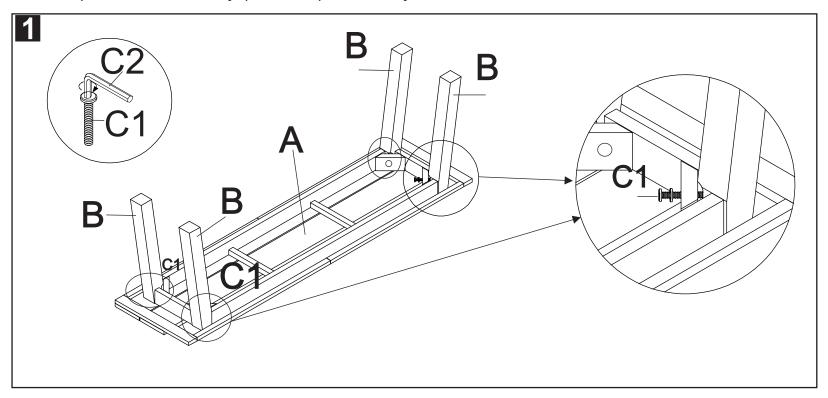
Step 1: attach the leg (B) to the seat (A) as shown on the picture. Using the Allen bolt (C1) and tighten all with the Allen Key (C2) as shown on the picture. Make sure all the Allen bolt is tighten before use.
