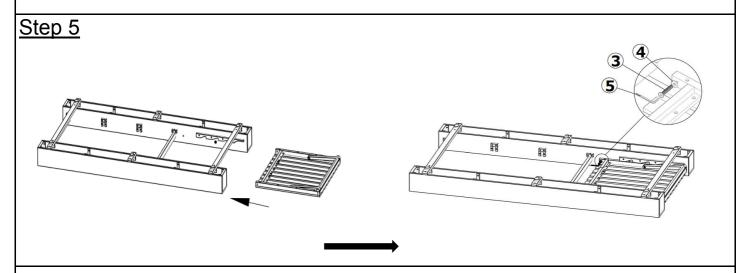
Attach the assemble in step 4 to assemble in step 2 using Bolts (3), Flat Washer (4) and Allen Key (5) as shown above
