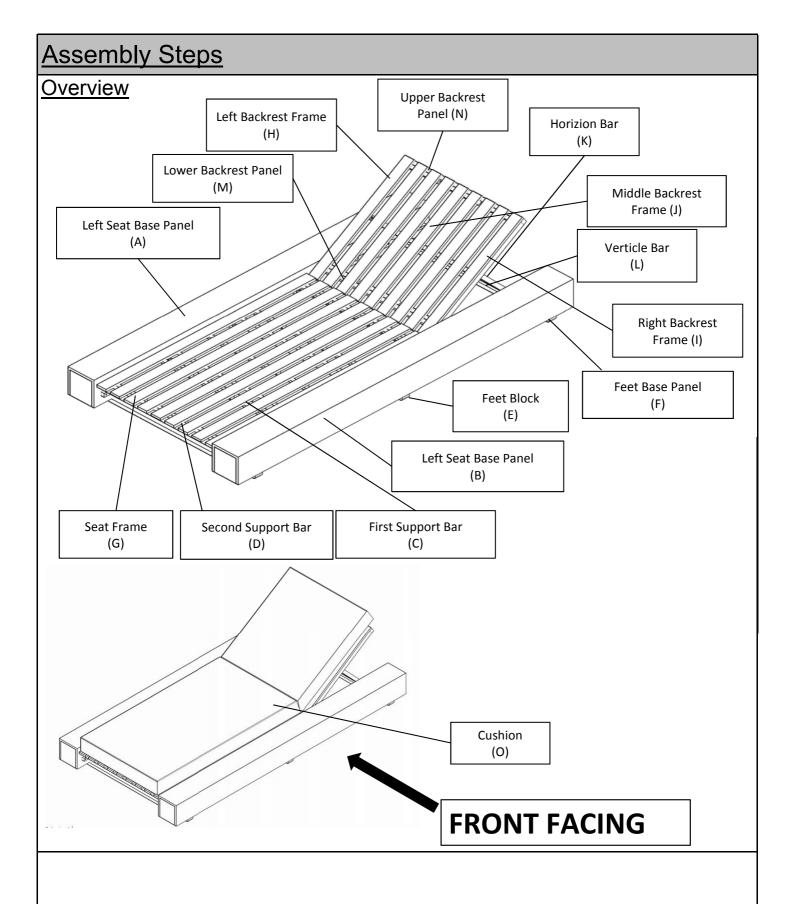
This Sun Lounger has multiple parts and may require up to 30 minutes to assemble. To give you an overview of the Bench, the above picture is to help you put the various parts into perspective. Please read through the instructions below to familiarise yourself with the parts and steps before assembly.
