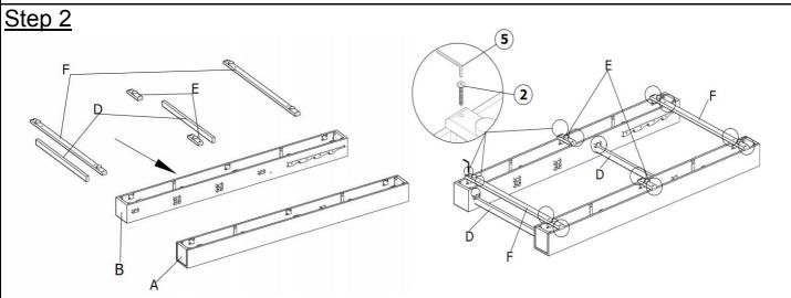
Position the Second Support Bar (D), Feet Block (E) and the Feet Base Panel (F) to the Left Seat Base Panel (A) and Right Seat Base Panel (B) using Screws (2) and (5) as shown above **Do not fully tighten the Screws**
