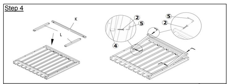
Attach the Horizion Bar (K) and Vertical Bar (L) to the assemble in step 3 using Screws ( $^{\circ}$ ) and Allen Key ( $^{\circ}$ ) as shown above
