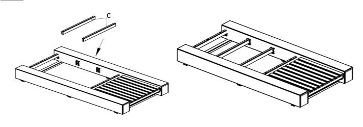
With the help of your adult partner, turn back the assemble in step 5 and attach the First Support Bar (C) to the frame as shown above
