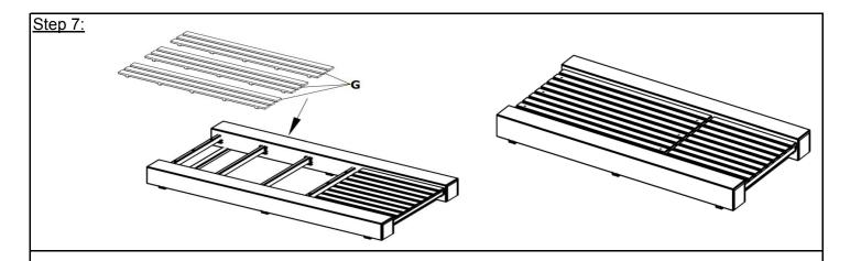
Position the Seat Frame (G) to the assemble in step 6 as shown above
