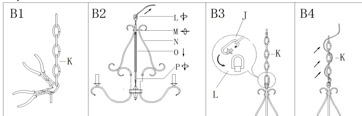
Step B1: By measuring, determine the correct number of links needed for proper hanging height. Using the chain pliers, disconnect and discard the remaining chain.
