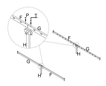
Attach Front & Rear Rail Section (F & G) to Headboard Leg (A), Headboard (B) and Footboard (C) using Bolt (O) with L-Allen Key (T).
