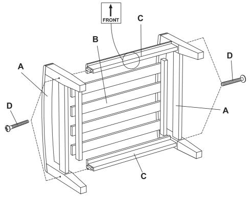
Attach the aprons (C) and stool (B) into leg frames (A) and secure using 2'' bolts (D). (Apron with round edge must attached in front )
