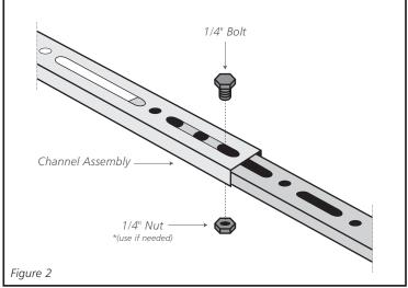
5. Thread the leveling bolts up through the holes in a pattern
