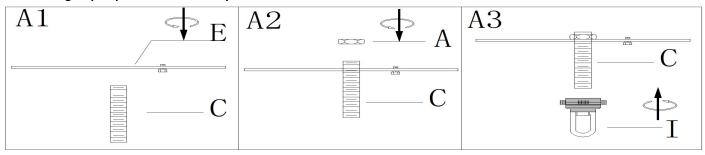
Step A1: Thread the single bar(E) over the nipple (C) a minimum of 6 mm (1/4"). At this point need note that: the side of
