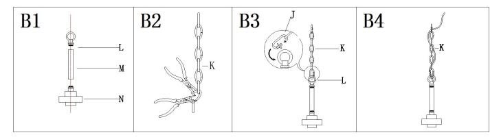
Step B1: Thread the tube (M)onto the top of lid till snug, and then thread the loop (L) onto the tube (M) till snug.
