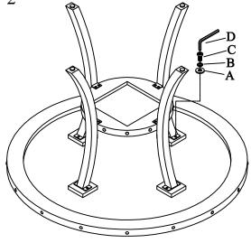
Do not tighten screws until completely assemboed
