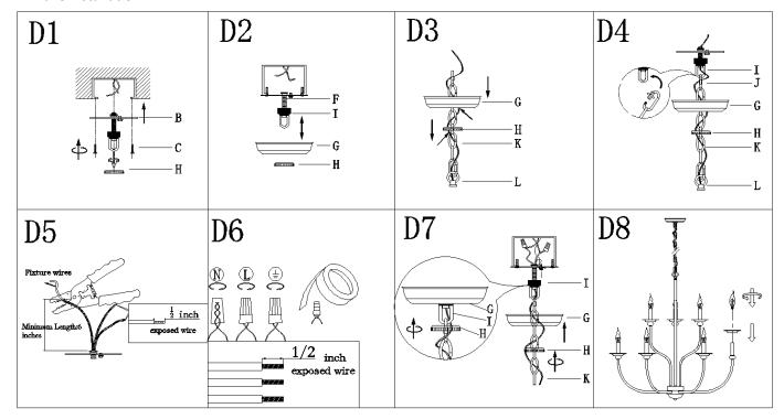
Step D1: .Attach single bar (B) to outlet box with mounting screw (C). The side of single bar marked "GND" must face out.
