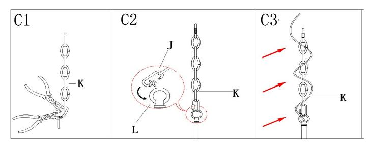
Step C1: By measuring, determine the correct number of links needed for proper hanging height. Using the chain pliers, disconnect and discard the remaining chain.
