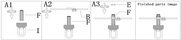
Step A1:Thread the nipple(F) into the screw collar loop (I) until it is tightly engaged within the screw collar loop (I).
