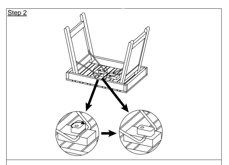
Rotate the Wooden Locks 90 degrees to lock Leg Supports into position.
