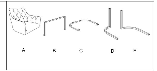
Place the Backrest (A), Support metal tube (B), Support rail (C), Left side tube (with Pre-attached Leveller) (D) and Right side tube (with Pre-attached Leveller) (E) on a clean, non-marring surface.
