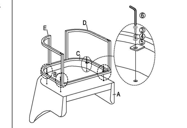
Attached Support metal tube (B), Support rail (C), Left side tube (with Pre-attached Leveller) (D) and Right side tube (with Pre-attached Leveller) (E) to Backrest (A) using Bolts(③), Washers(④), and Spring Washer(⑤) with Allen Key(⑥) as shown in above picture.
