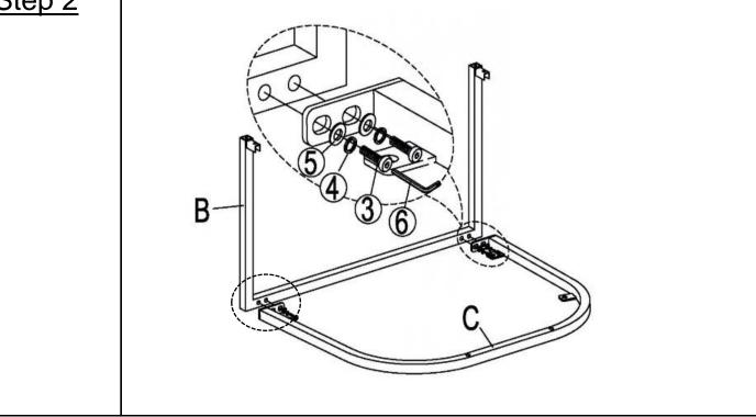
Attached Support metal tube (B) to Support rail (C) using Bolts(3), Washers(4), and Spring Washer(5) with Allen Key(6) as shown in above picture.
