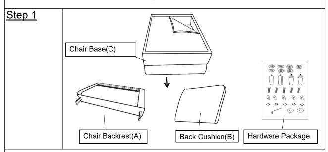
Put the Chair Backrest(A) facedown on a clean, non-marring surface. Uncover the non-woven Fabric and remove Chair Backrest(A), Back Cushion(B), and Hardware package from Chair Base(C).
