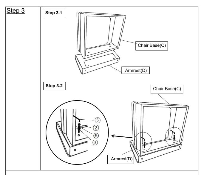
Step3.1 Position Chair Base(C) and Armrest(D) upside down on a flat surface. Step3.2 Attach Chair Base(C) to Armrest(D) ,using Bolt(2), Washer Ring(6), Washer(3) with Allen Key(5) until tight. Repeat the same step to install remaining Armrest(D).
