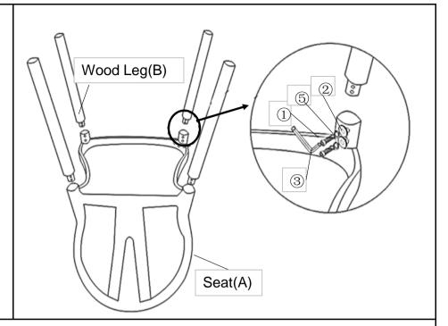
Place the Seat(A) face down, on a clean, non-marring surface. Insert the Wood Leg(B) into Seat(A), align mounting positions between the Wood Leg(B) and Seat(A), then attach the Wood Leg(B) to Seat(A) using Bolt(1), Spring Washer(5), Flat Washer(2) with Allen Key(3).
