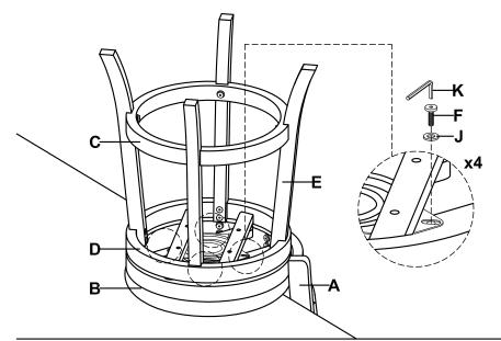
Stand the chair on an even surface and check for balance. If it wobbles, apply downward pressure on the uneven leg and tighten the bolts. Once the chair is balanced, apply pressure evenly to the center and tighten all bolts, ensuring not to over-tighten beyond the hole depth.
