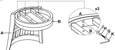
Keep the Backrest (A) and Cushion Seat (B) inverted on the surface. Attach the swivel plate on the Apron (D) to the Cushion Seat (B) using Bolt (F) and Flat Washer (J) with Allen Wrench (K).
