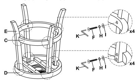
Take the Allen Wrench, and turn the bolts until the legs are secured. DO NOT TIGHTEN COMPLETELY. Stop when you feel you are adding force to tighten the bolt.
