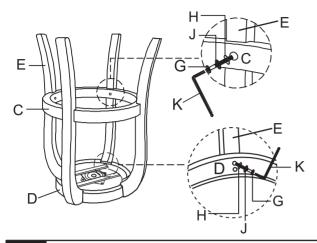
Take the Allen Wrench, and turn the bolts until the legs are secure. DO NOT TIGHTEN COMPLETELY. Stop when you feel you are adding force to tighten the bolt.
