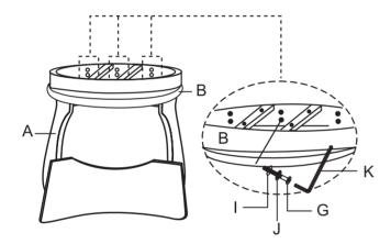
Keep the Backrest (A) and Cushion Seat (B) inverted on a stable raised surface. Attached the Swivel Plate located on the Apron With Swivel Plate (D) to the Cushion Seat (B) using Bolt (F), Flat Washer (I) with Allen Wrench (K). Turn the Swivel Pub Stool right side up.
