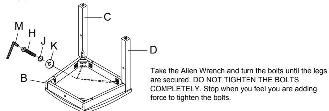
While placing the Left & Right Stretcher (E & F) between the front and back legs, attach the Seat (B) to the Back Frame (A) by using Bolt (G) (corners) and Bolt (I) (center), along with Lock Washer (J) and Flat Washer (K) with the Allen Wrench (M).
