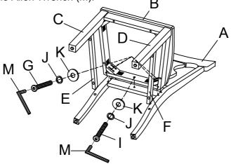
Fix the Left & Right Stretcher (E & F) to the legs by using Screw (L) with a screwdriver (not provided).
