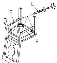
Stand the chair on an even surface and check for balance. If it wobbles, apply downward pressure on the uneven leg and tighten the bolts. Once the chair is balanced, apply pressure evenly to the center and tighten all bolts, ensuring not to over-tighten beyond the hole depth.
