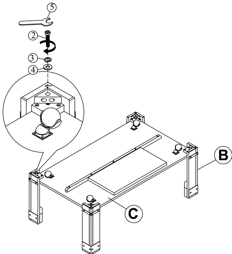
STEP 2 : Place the Table Top (A) on its side as picture shown. Make sure the Top opened in the opposite direction to the heavy panel underneath the bottom panel in order to keep the table on balance . Open the top panel and attach the assembled base in Step 1 to the Top by using Flat Washer (4) Lock Washer (3) and Long Bolt (1) through the corner block. Secure well by Wrench (5). Fully tighten all the bolts at this time. Assembly product is now completed.
