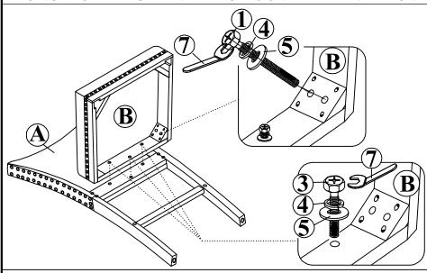
Step 1: Place the Chair Back (A) on the floor. Attach Seat Box w/Seat Cushion (B) Chair Back (A) by inserting the Flat Washer (5), Lock Washer (4), Short Bolt (3) into the holes at the rear bar of the seat frame. Insert Flat Washer (5),Lock Washer (4), Long Bolt (1) into the holes at the corner block of the seat box. Tighten all Bolt with Open Wrench (7). Do not fully tighten.
