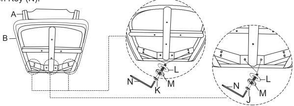
Keep the Backrest (A) and Cushion Seat (B) inverted on a stable raised surface. Attached the Swivel Plate located on the Apron with Swivel Plate (E) to the Cushion Seat (B) using JCBC Screw (I), Flat Washer (L) with Allen Key (N). Turn the Chair right side up.
