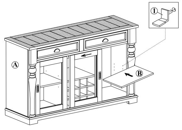
Step 2: Place the Server (A) on flat surface and adjust the Leveler until level and does not wobble.
