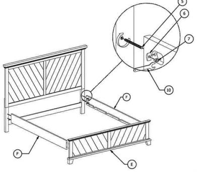
Step 3: Insert the long drat (5) into the assembly headboard and footboard (E), tighten all long drat at this time. Then assemble side rail to headboard and footboard using halfmoon (6), lock washer (7) and hex nut (8) as picture shown, tighten with wrench(11)
