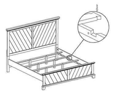
Step 5: Attach the assembly slat with middle leg into the groove on the side rail. assembly product is now completed.
