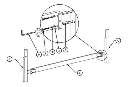
Step 1: Place all parts down on a piece of cloth or carpet to prevent finish from scratching. insert the wood dowel (9) to the bottom support (B) and then assemble with leg (C) & (D). insert machine screw (1), lock washer (4), flat washer (3) into the hole. tighten with allen key (10)
