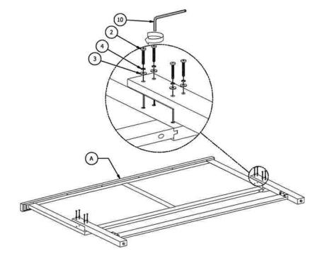
Step 2: Attach assembly bottom support with leg into the panel headboard(A). insert the machine screw(2), lock washer (4), flat washer (3) into the hole, tighten with allen key(10)
