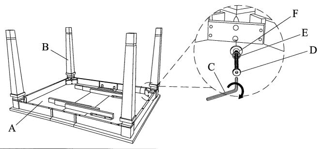
2 Flip table over using two people to lift and flip the table. Unlock the latches underneath table top(A). Pull apart the table top(A) at both ends and take out the center leaf.
