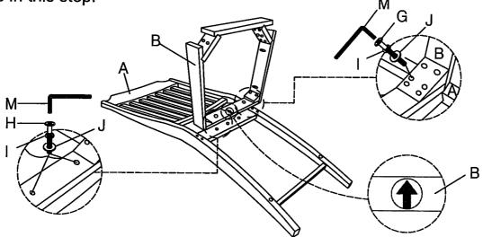
Take the Allen Wrench, and turn the bolts until the legs are secured. DO NOT TIGHTEN COMPLETELY.
