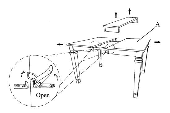
Push both ends together and make sure pin line up. Close the table top(A) tightly and lock all latches on the underneath of the table.
