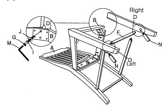
4 Insert Pan Head Screw (L) into the holes of Front Leg (D) and Stretcher (F) by using Screwdriver (not included).
