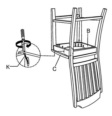
Turn the assembled chair to the upright position carefully. Make sure the chair is level, and then securely tighten all bolts at this stage. Assembly is now completed.
