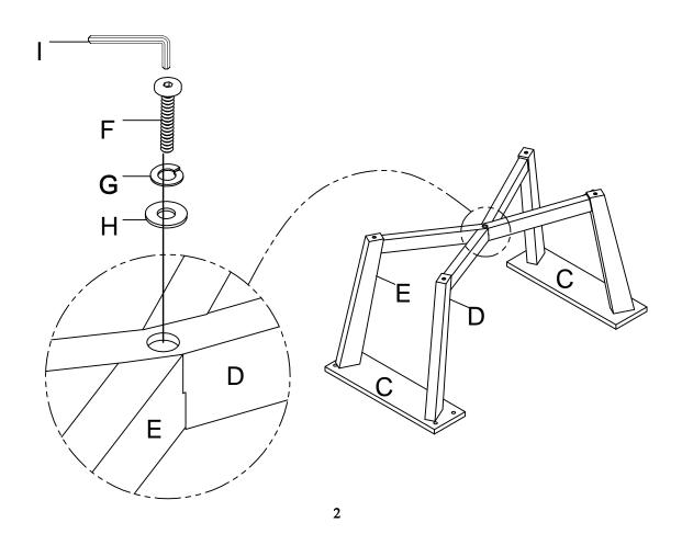
Attached Mounting Plate(C) to the Table Top(A). Use Allen Bolt(F) Lock Washer(G) and Flat Washer(H) on holes of Table Top(A). Turn the Allen Key(I) in Allen Bolt(F).
