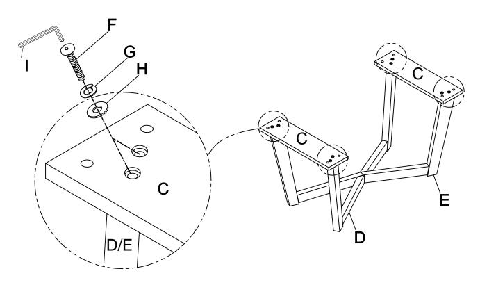
2 Use Allen Bolt(F) Lock Washer(G) and Flat Washer(H) on holes of Leg Down(D). Turn the Allen Key(I) in Allen Bolt(F).
