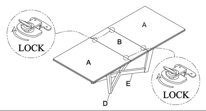
Adjusted the Leveler at the bottom of Leg(D,E), to keep the table level.
