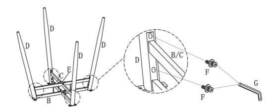
Place Table Top (A) upside down on a stable, smooth and carpeted surface. Then, attach Table Leg (D) to Table Top (A) using Bolt with Lock Washer and Flat Washer (F) with Allen Wrench (G).
