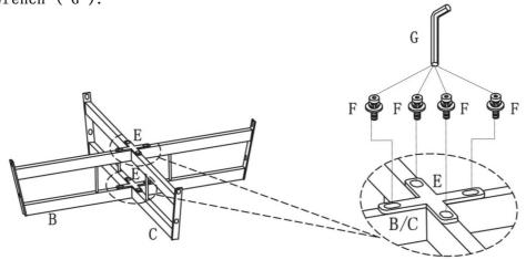
Align and attach Table Leg (D) to the assembled frame (B & C) using Bolt with Lock Washer and Flat Washer (F) with Allen Wrench (G).
