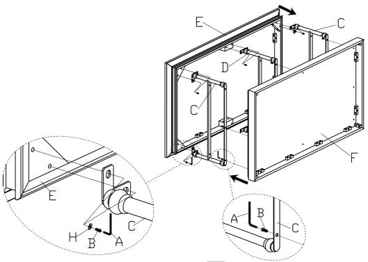
Assembly the Shelf(G) onto the Side Frame(C) and using the Bolt(B) by Allen Wrench(A).
