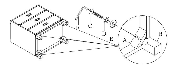
Attach Anti-tipping hardware(G) to wall: Attach bracket (vertically) to wall using 2 of the screws provided; Attach bracket (horizontally) to furniture back (directly below top) with 2 of the screws provided. Place bracket as close to center of furniture back as possible in relation to wall stud and the desired position in the room; Move furniture to its final position. Thread the strap through bracket, pull it tight.
