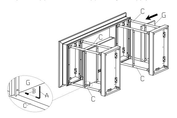
Assembly the Cross Bar(D) onto the Side Frame(C) and using the Bolt(B) by Allen Wrench(A).
