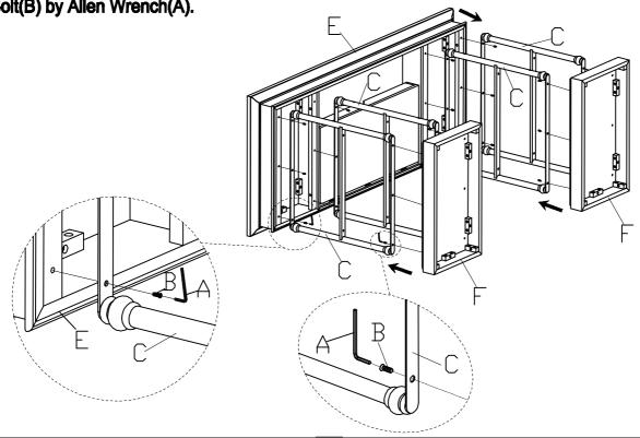
2 Assembly the Shelf(G) onto the Side Frame(C) and using the Bolt(B) by Allen Wrench(A).
